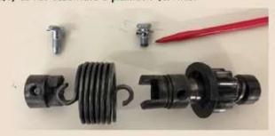
The other bolt is "special" only because it is only 11/16" long. This allows the bolt to lock the spring in place, without having the bolt actually touch the starter shaft. Don't be tempted to use a 3/4" long bolt instead of the correct shorter one. See the comparison photo of a 3/4" bolt and the correct bolt.
